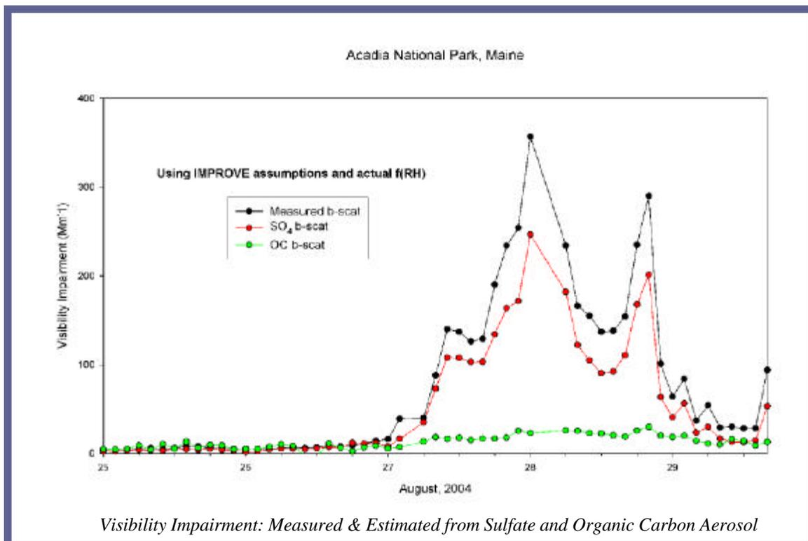
RAIN monitors gather particle mass, composition, and optical property measurements every 1-2 hours to provide enhanced insight into regional aerosol generation and source characterization, factors that drive short-term visibility, and aerosol model performance and evaluation.
