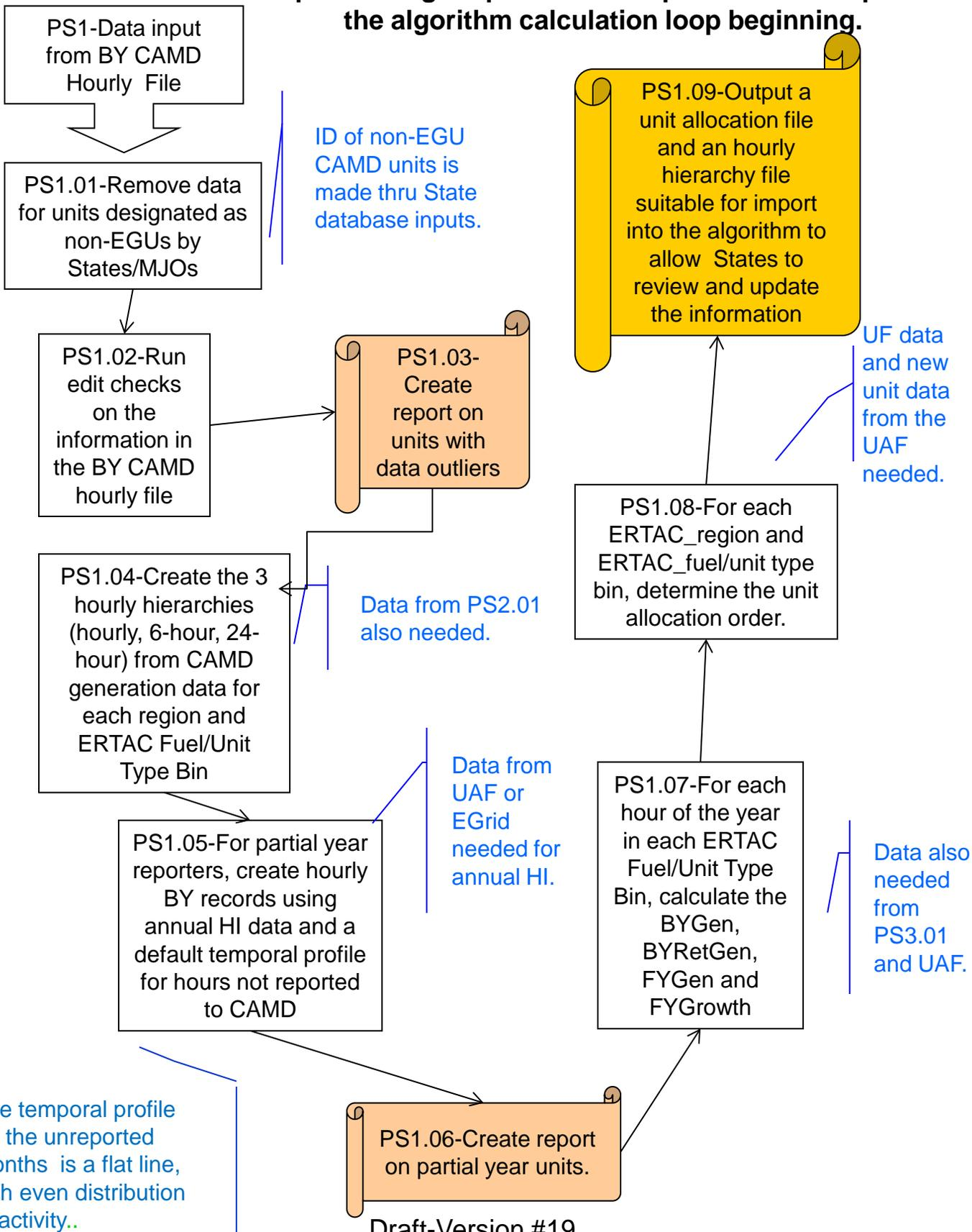
**Preprocessing Steps: These steps can be done prior to the algorithm calculation loop beginning.**
